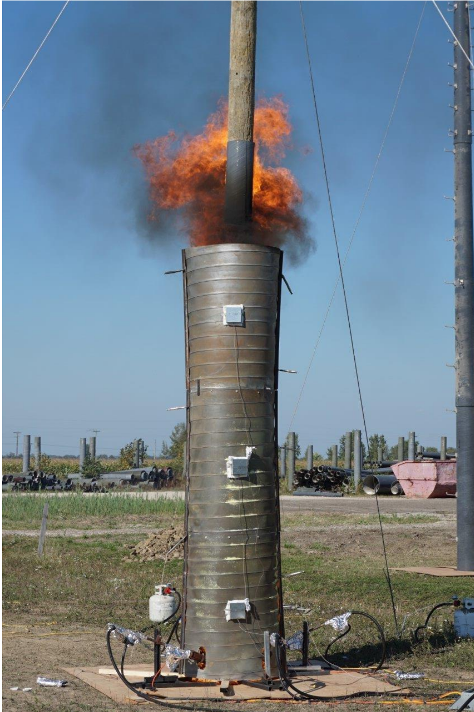
35 ft. [10.7m] Red Pine Wood Pole with RS Fire Shield™ Fire Test, 2-Minute (Severe) Exposure
