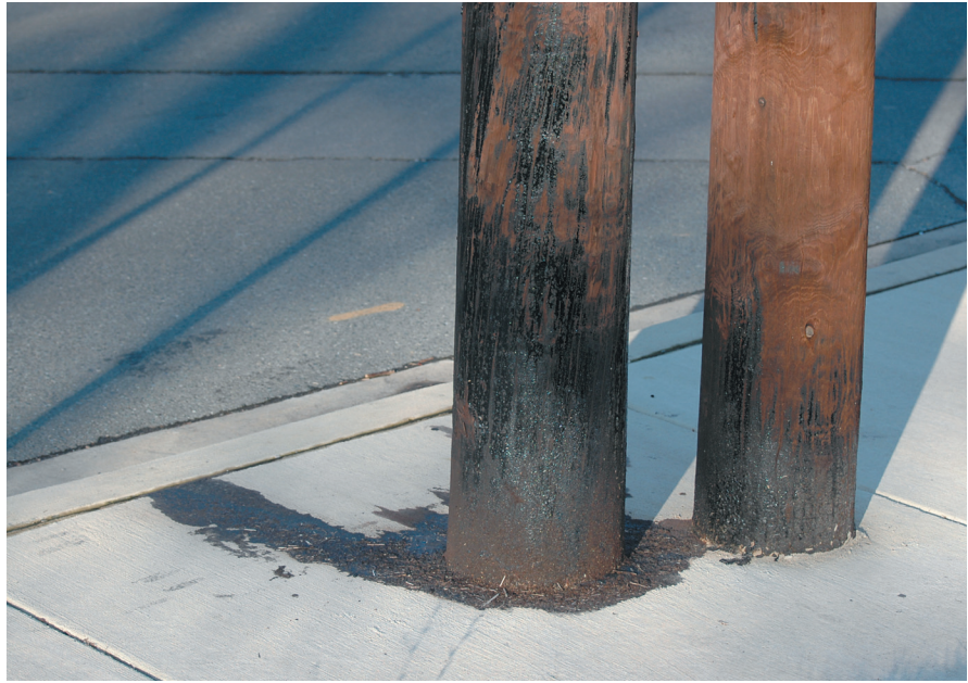
Environmental regulations now consider treated wood poles as hazardous waste.
